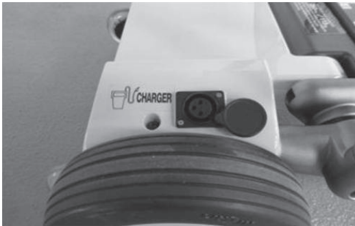
battery charging Port
